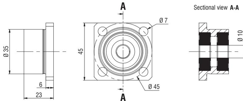
Flange bearing floating bearing end
