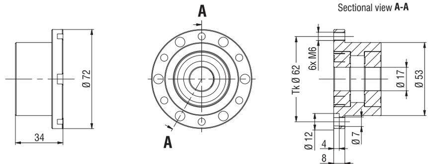
Flange bearing floating bearing end
